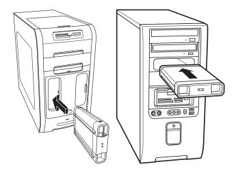
To insert the HP Personal Media Drive into a specially designed HP PC:
