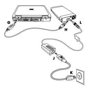
**5** Plug the rectangular end of the USB 2.0 cable (**G**) into an available USB port on your PC. Plug the square end of the USB 2.0 cable (H) into the USB connector on the back of the drive.
