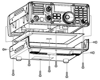
③ Replace the circuitry fuse as shown in the diagram as below.
