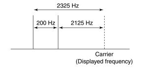
The RIT (Receive Incremental Tuning) function compensates for stations transmitting off-frequency or when you prefer to listen to slightly different-sounding voice characteristics, etc.
