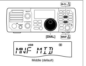
While adjusting the manual notch filter, noise may be heard. This comes from the DSP unit and does not indicate an equipment malfunction.
