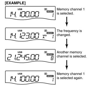
Changed frequency (14.123 MHz) does not appear and memorized frequency (14.100 MHz) appears instead.
