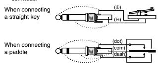
If you use an external electronic keyer, make sure the output voltage of the keyer is less than 0.4 V when keying the transmitter.
